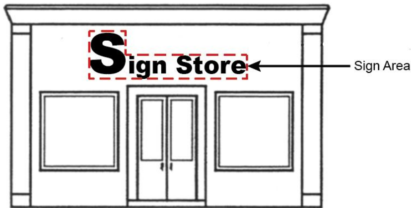
Figure 8-D: Illustration of sign area calculation for two differently shaped wall signs with individual letters.
